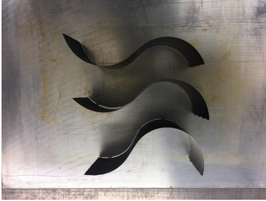
Figure 1: Example of curved laminates made by 4D printing
