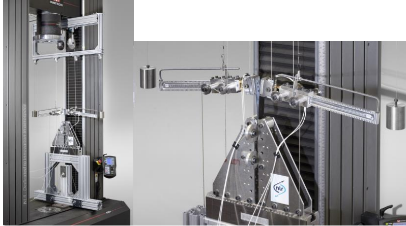
Figure 9: Moment loading cantilever beam setup. This will enable a-symmetric coupons to be testing in Mode I, Mode II and mixed modes with constant moment. The load is applied by the arms which are loaded by the steel cables.
