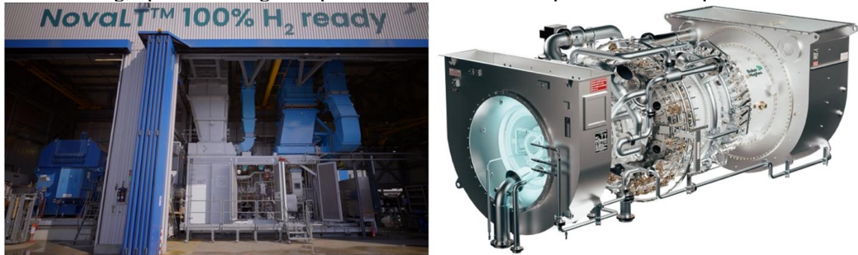
Figure 1: Left: NovaLT™ 100% H 2 ready gas turbine, installed on the Baker Hughes test bench at Florence site (IT). Image courtesy of Baker Hughes. NovaLT™ is a trademark of Baker Hughes and its affiliates. All right reserved.
