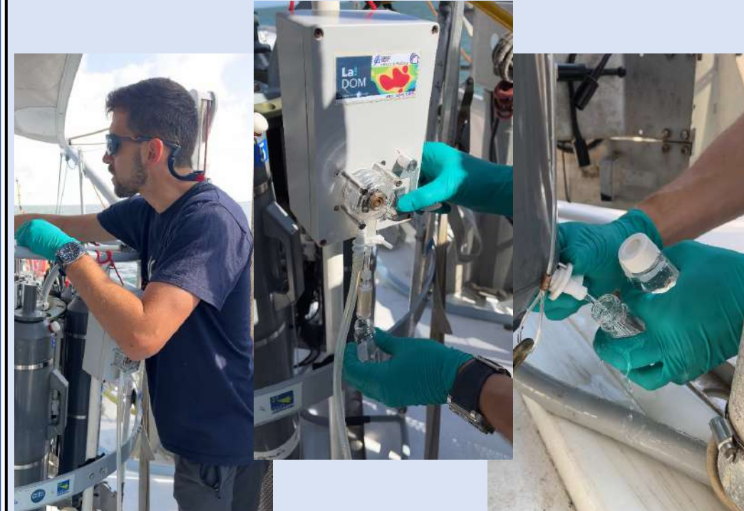
Filtration with a portable pump attached to the niskin
