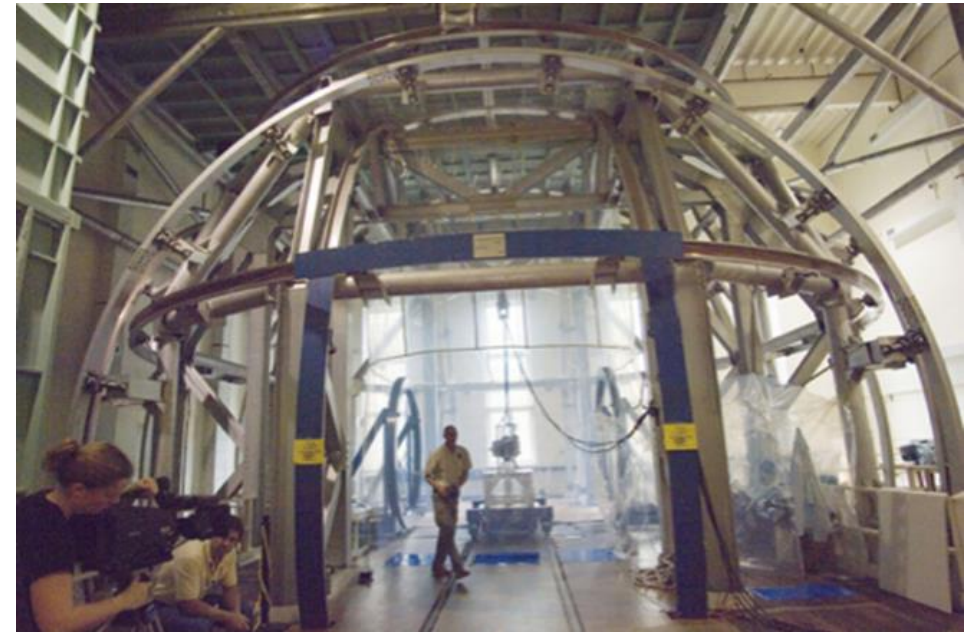
A view inside the magnetic coil facility at (Goddard Space Flight Center) GSFC. Coils are 42 ft in diameter with the ability to produce an 8-ft diameter region of homogeneous magnetic field that is stable and accurate to within \pm 0.25 nT. Another set of coils cancels the Earth’s local magnetic field.
