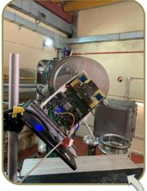
Special setup to account for target cooling beam shaping Passive irradiation of SiPM for displacement damage test on silicon, with different fluences
