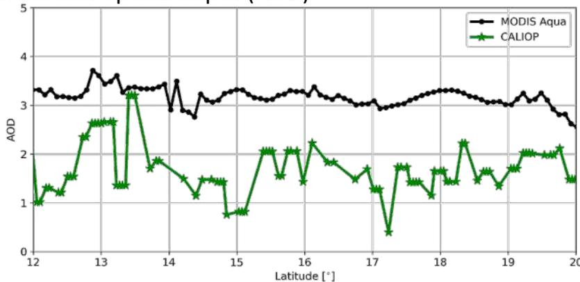
CALIOP underestimates AOD (CALIOP measurements with attenuated bins have been removed)
