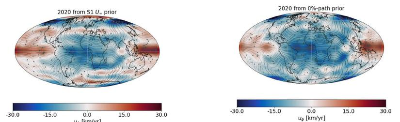
Main features reproduced: e.g. eastward flow under the Equatorial Pacific
