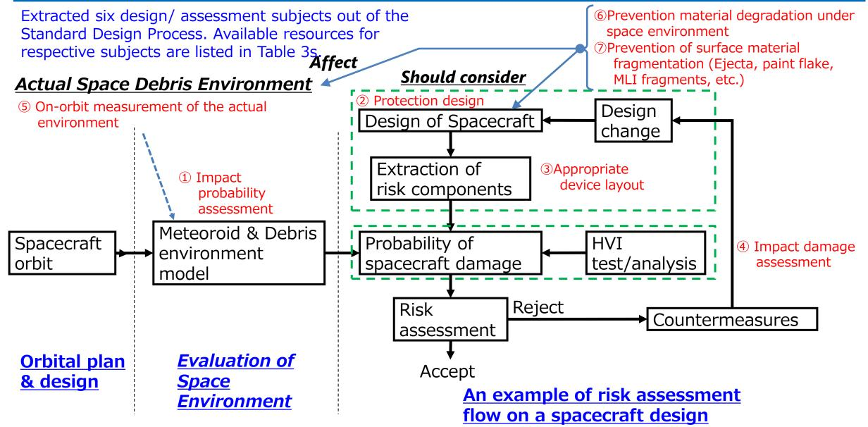
Modified and simplified flow based on JERG-2-144 Micro-debris Impact Survivability Assessment Procedure (Kitazawa, et al., 2016) 31
