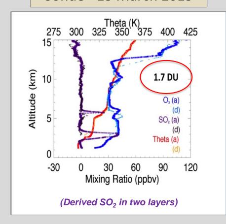
Tropospheric column derived from the dual sonde technique\* is 1.7 DU SO<sub>2</sub>. Sonde column in excellent agreement with single, co-located OMI PCA pixel.
