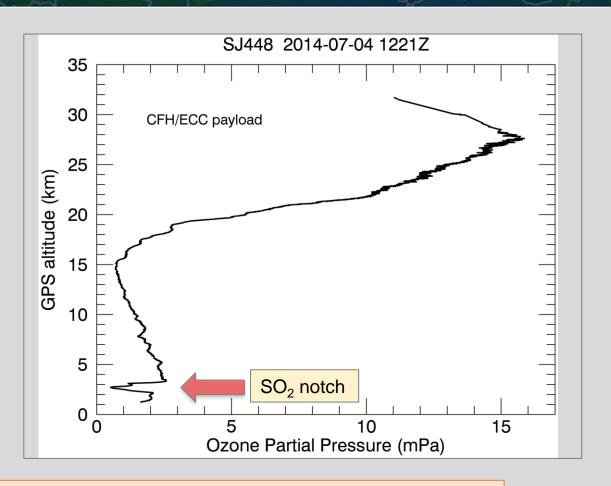
Since 2005, layers of SO<sub>2</sub> have appeared as interference notches in ozone profiles launched from the successive Ticosonde sites at Alajuela, Heredia and San Pedro. All are located downstream of Turrialba and the notches are due to SO<sub>2</sub> emitted from the volcano.
