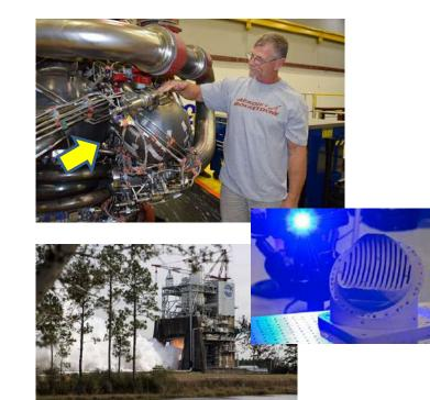
RS25 Prime Contractor, Aerojet Rocketdyne, technician exhibits the RS-25 pogo accumulator (top and middle), which was subsequently hot-fire tested (bottom)
