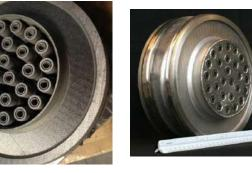
28-element Inconel<sup>®</sup> 625 fuel injector built using a laser powder bed fusion (L-PBF) process
