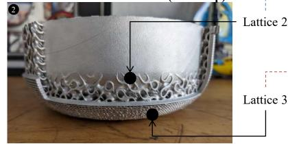
Hexagonal Honeycomb (Internal Stiffness)
