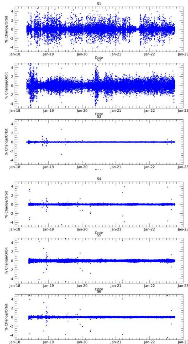
Using time-series of calibration signals we can estimate orbit-orbit stability of each channel
