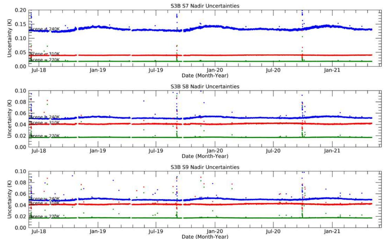
Uncertainties derived from analysis of L0 data from Instrument Temperatures, BB signals, Gain-Offset variations, Noise...
