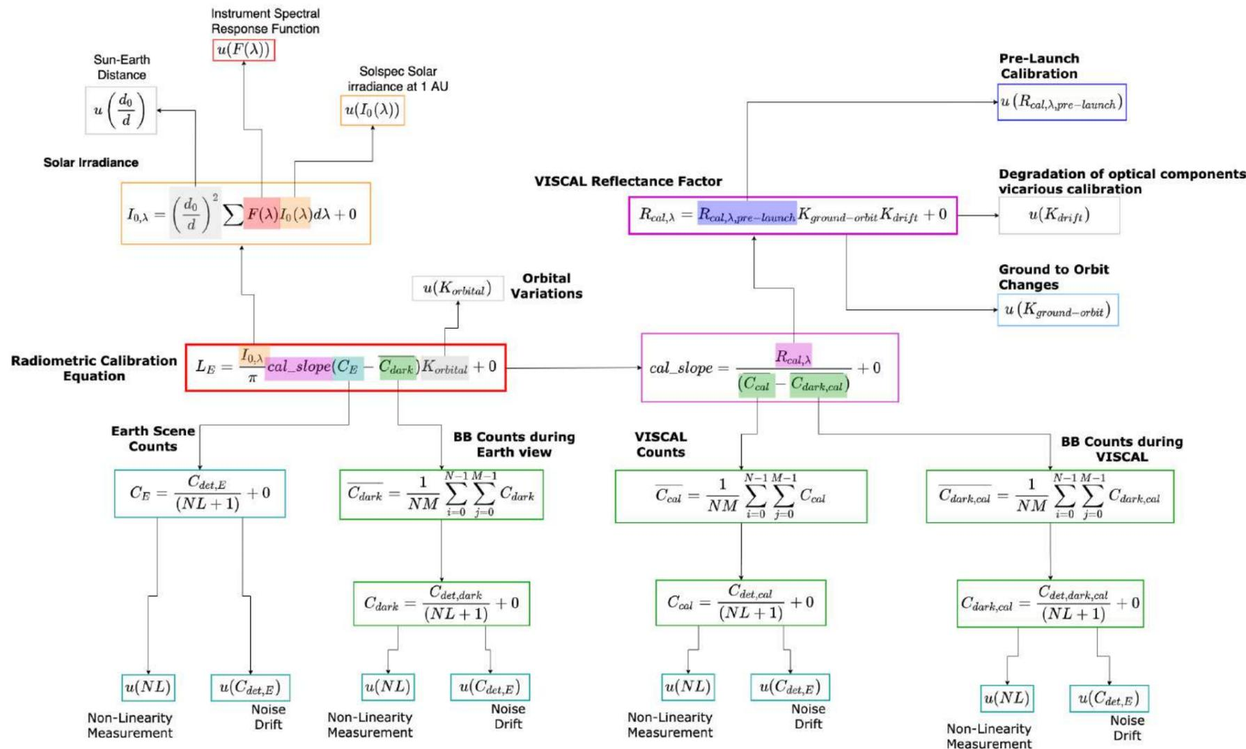
We can propagate further to examine effects due to changes between ground-to-orbit of optical chain:
