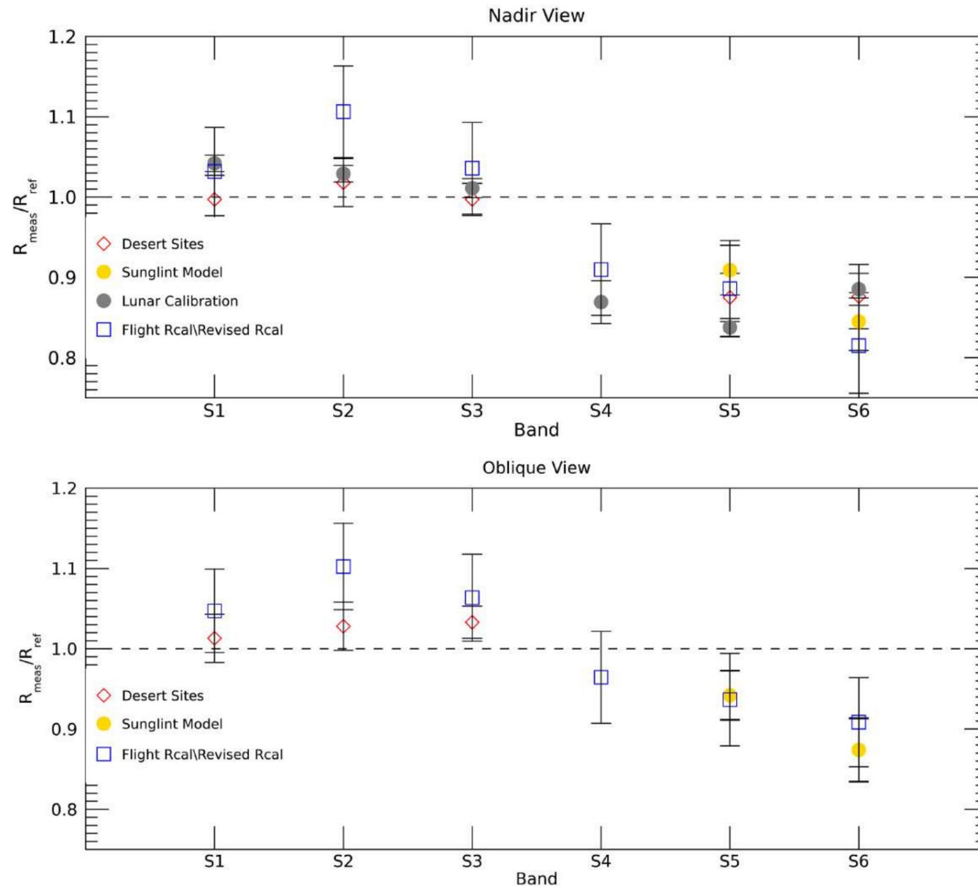
Reprocessed SLSTR-B pre-launch calibration factors are consistent with the vicarious calibration measurements within uncertainties
