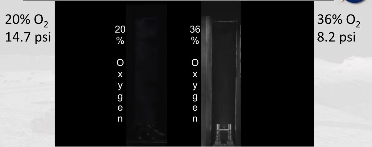
Due to desired properties of cotton, it will likely be used for underwear and towels. Though flammable in air, ignition and propagation occurs more readily in oxygen-enriched exploration atmospheres. Susana Harper, White Sands Test Facility
