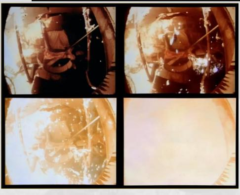
In a **post Apollo I mockup test**, fire spreads rapidly through the command module cabin in pure oxygen at 16.7 psi
