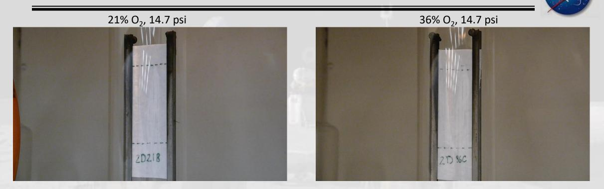
Ignition time and flame spread occur rapidly at 36% oxygen.
