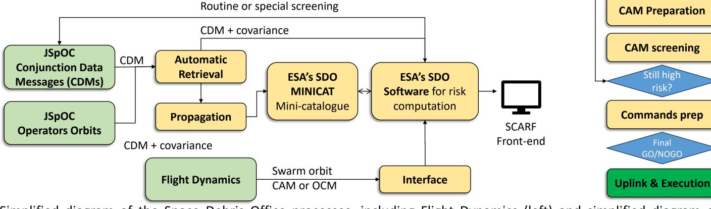
Simplified diagram of the Space Debris Office processes, including Flight Dynamics (left) and simplified diagram of the Collision Avoidance Management process at ESOC for a given mission (from Warning to CAM uplink and execution (right).
