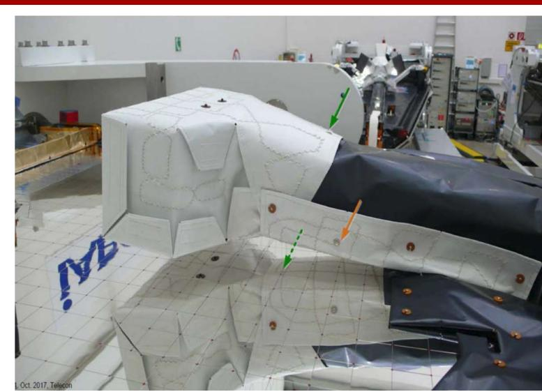
which are electrically connected both through the grounding network as well as through the thermal blankets, hence currents will flow in the blankets and grounding wires in close proximity to the magnetometers. The differences in the estimated  $dB_Sun$ 's (cf plots at the bottoom of this poster) of the three spacecraft can be explained by differences in resistances, mainly contact resistances and resistances in the aluminum foils of the thermal blankets.
