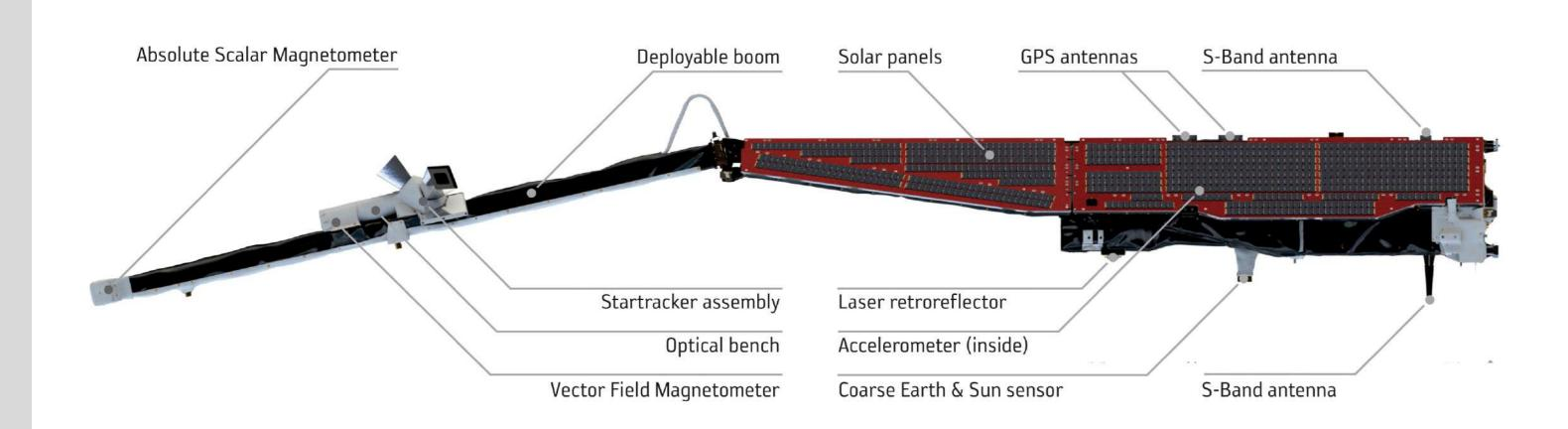
The two science magnetometers on Swarm are the Absolute Scalar Magnetometer (ASM) at the tip of the boom and the Vector Field Magnetometer (VFM) 1/3 inwards on the boom. Around both magnetometers are the white, thermal blankets made of an outer layer of betacloth and multiple aluminum layers beneath. Also noticeable is the thermal blanket on the bottom side of the boom, a.k.a. the "boom-blanket".
