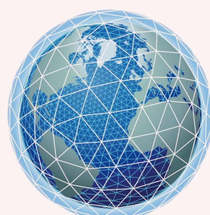
Scheme of the ICON unstructured triangular grid
