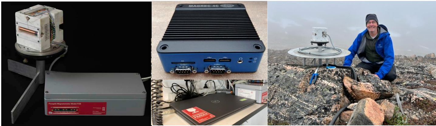
Instrumentation: Magnetometer, for example 3-axis Fluxgate Magnetometer Model FGM – FGE built by Lars W. Pedersen and Jan Oechsle. Data loggers example to the right, windows laptop, and Linux magrec datalogger from MinGeo.
