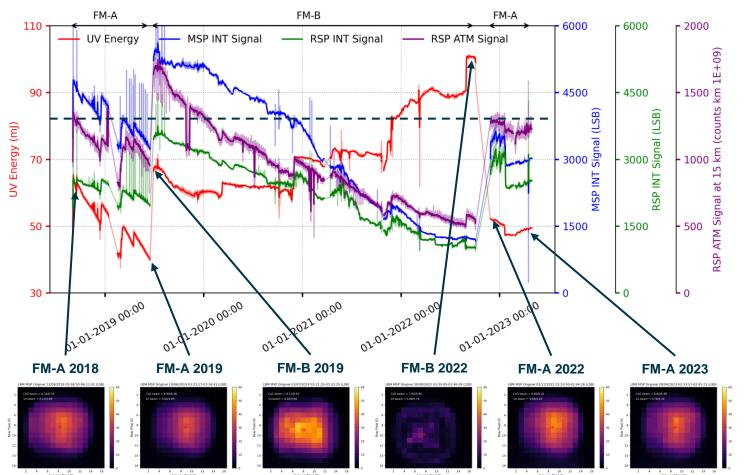
Long term evolution of several ALADIN signal levels (PD74 UV energy, INT path signals, and the Rayleigh ATM path signal at 15 km) over the Aeolus operational mission and the NF beam profiles.
