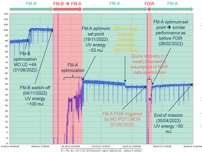
Laser UV output energy from the end of FM-B, switch-back to FM-A with main events towards the end of the operational mission lifetime.
