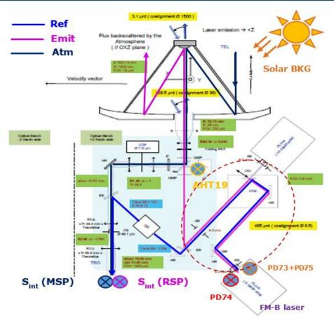
Schematic of the ALADIN instrument indicating the optics impacted by optical attenuation (red ellipse)
