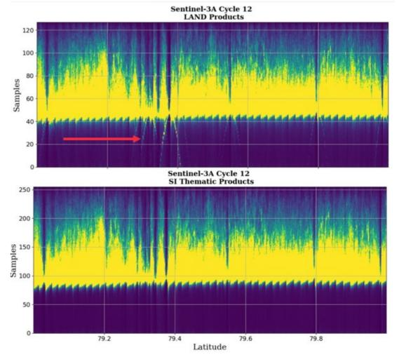
Example of the impact of the Hamming weighting for specular echoes
