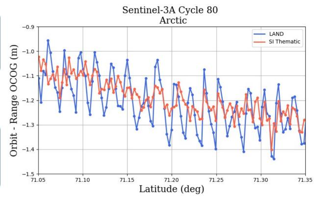
Reduction of the jitter noise on S3 thanks to the zeropadding,
