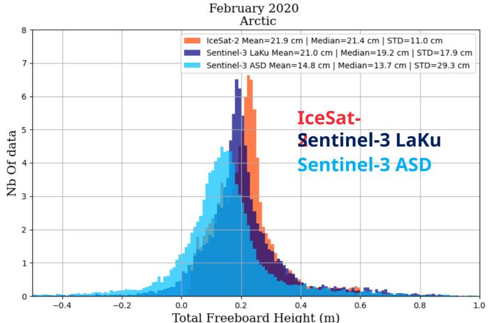
**1cm** mean bias with snow LaKu **7cm** mean bias with snow ASD Several differences between IceSat-2 ATL10 and S3 processing : → For instance : IceSat-2 freeboards < 0 are edited
