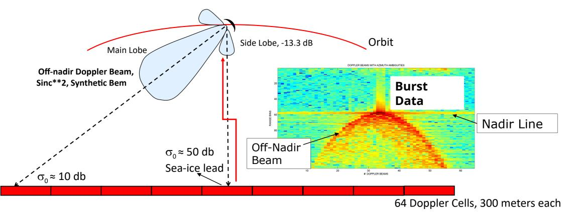
At burst Level, spurious returns show up as "straight line" . At stack level (i.e. after the range migration), the straight-line artifact will become "parabolic arch" To suppress parabolic arches on the waveforms => application of a weighting window to the burst data <u>in azimuth dimension</u> before the Beam-Forming. In this slide, weighting window is Hamming window
