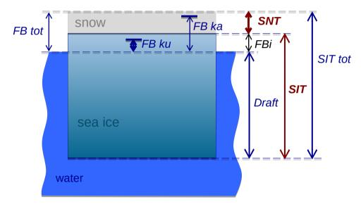
Wanted parameters: sea ice thickness SIT snow thickness SNT Intermediate parameter: ice freeboard FBi
