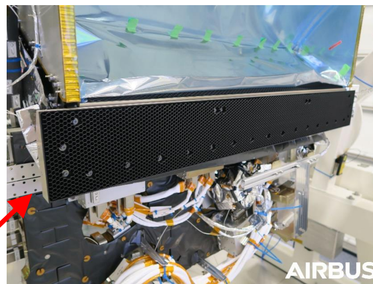
SWIR cold box (black) SWIR focal planes/detectors (foreground), tied to the cold radiators by gold thermal straps
