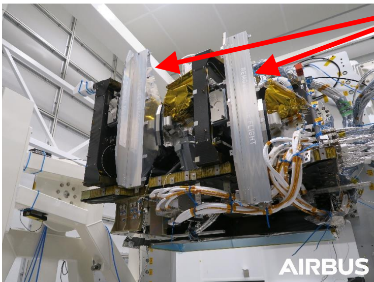
US and VN telescopes, (with covers), UV1 (middle), FEE (bottom)
