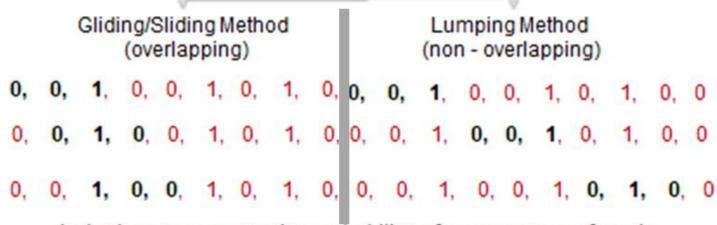
In both cases, count the probability of appearance of each "block of length m" and compute the block entropy H(m).
