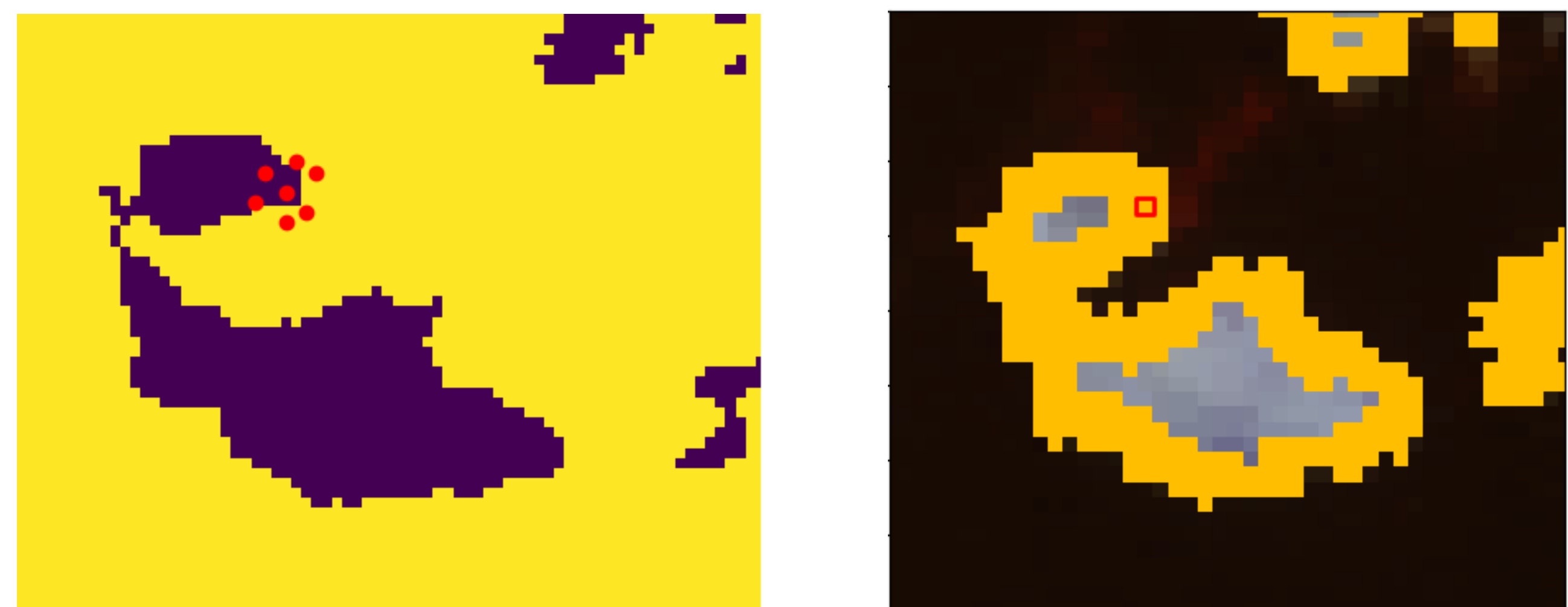
Fig 3. The vertices of a single pixel are shown by the red dots in the image above, where ocean is yellow, and land is purple. We see that three vertices and the central pixel are land, and the other four are ocean. Therefore this pixel is classified as coast.
