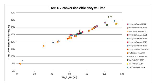
TxA FM-B UV Conversion Efficiency in vacuum versus UV energy, starting from TxA test campaign to Oct 2022 in-flight
