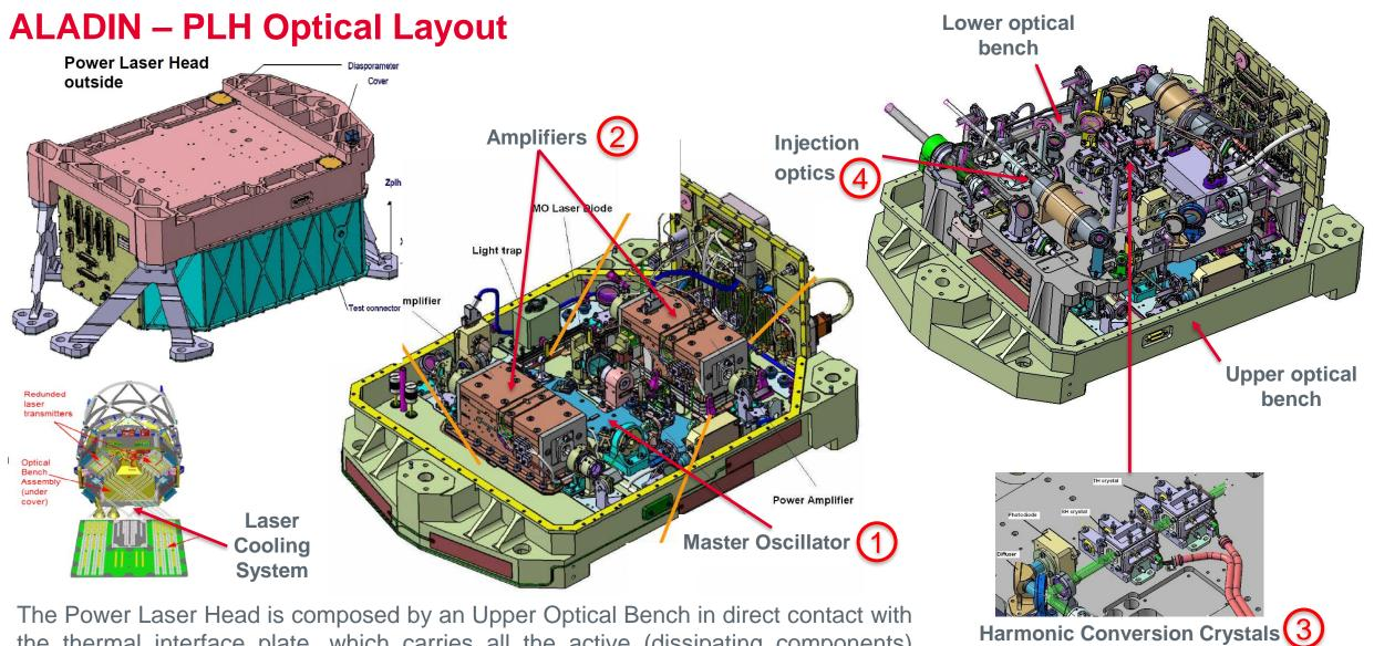
The Power Laser Head is composed by an Upper Optical Bench in direct contact with the thermal interface plate, which carries all the active (dissipating components) Passive components are located on a separated Lower Optical Bench
