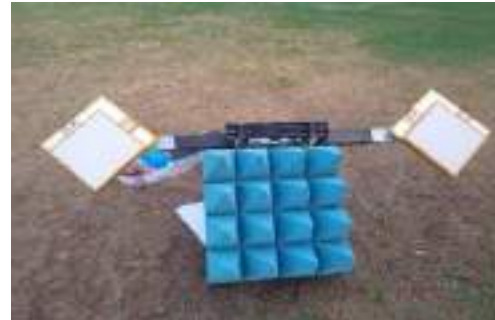
Indigenously developed Wideband Active Radar Calibrator (ARC) (L, S, C & X band)
