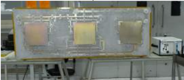
1.5m x 0.5m Antenna to mounted in belly
