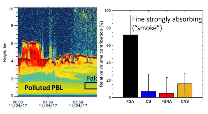
Optical Properties at 1.2 - 1.5 km height (355, 532 nm) Lidar Ratio (sr)  $67 \pm 13$   $66 \pm 32$ Depolarization Ratio  $12 \pm 2\%$   $4.5 \pm 2\%$
