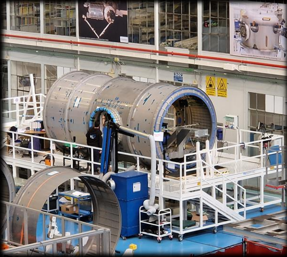
HALO primary structure, currently under static test (on foreground forged cylinders of I-HAB)
