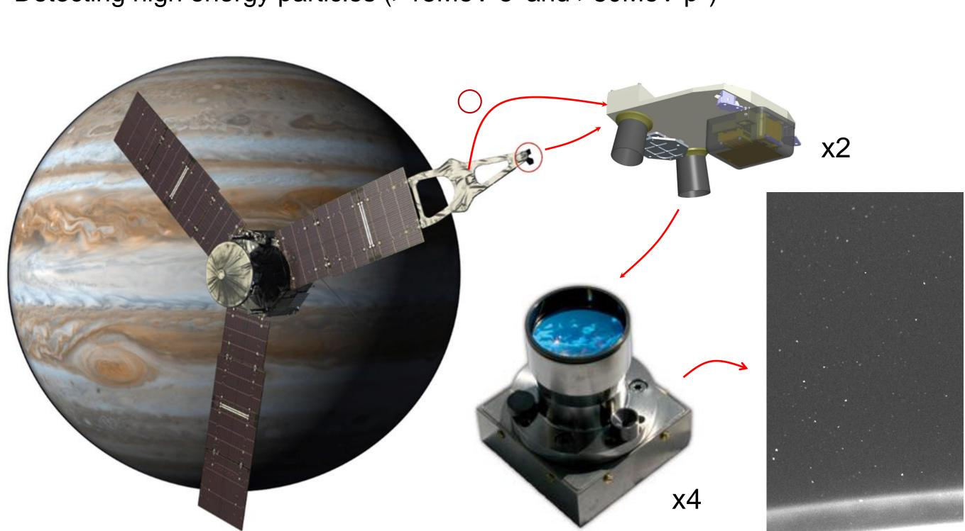
Figure 1: microASC cameras on the Juno MAG investigation optical benches. Image Credit NASA, DTU
