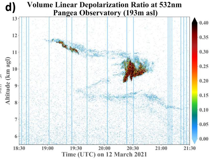
Ash concentrations **a,b)** w/w-o Aeolus assimilation, **c)** the time-height curtain plot of the attenuated backscatter coefficient and **d)** volume linear depolarization ratio based of **Polly<sup>XT</sup>-NOA lidar retrievals** at the PANGEA station during **12 March 2021 (18:30 to 21:30UTC)**.
