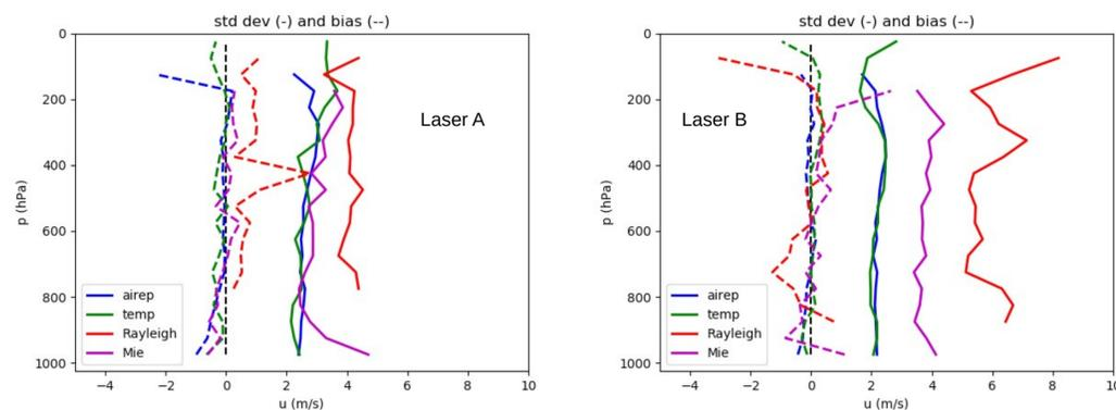
Fig. 2: Standard deviation and bias of O-B for Aeolus Mie (purple lines) and Rayleigh (red lines) HLOS winds compared to radiosondes (green lines) and aircraft data (blue lines).
