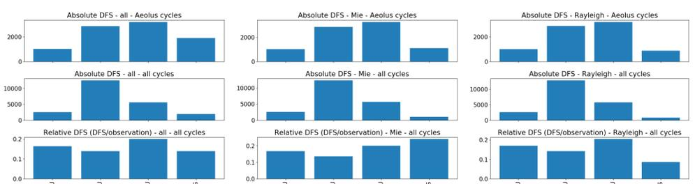
Fig. 4: Degree of Freedom of Signal (DFS) for the laser B period comparing Aeolus winds with SYNOP, radiosondes and aircraft data.
