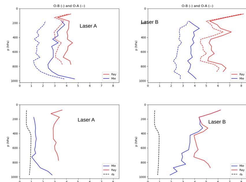
Fig. 3: Top row: standard deviation and bias of O-B and O-A for Rayleigh (red lines) and Mie (blue lines). Bottom row: Mean observation error and background error.
