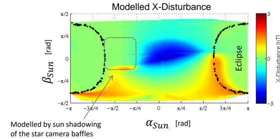
The distribution of the x-axis disturbance is similar on all three Swarm satellites indicating similar perturbation mechanism. However, disturbance in the y-axis is somewhat different. On the y-axis the perturbation seem to be induced by the sun coming for above the satellite (not from the side).
