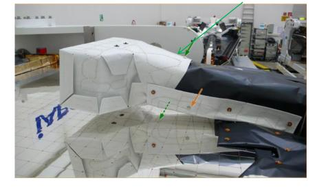
The ASM thermal blanket is designed similar to the VFM blanket but the rivets are placed up/down and the shape of the MLI blanket argues for a y-axis disturbance. The y-axis disturbance of the ASM has later been confirmed by intersatellite comparison of the ASM magnetometers on the two spacecraft's.
