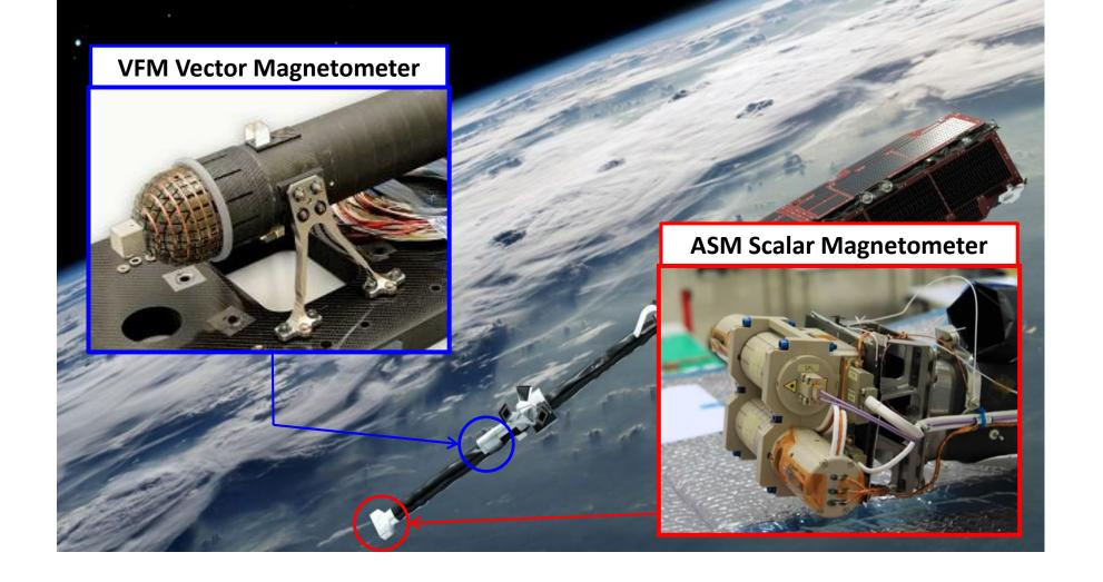
The planned in-flight calibration scheme was to adjust the sensitivities, offsets and orthogonality angles (9 parameters) of the VFM to minimize the scalar residual
