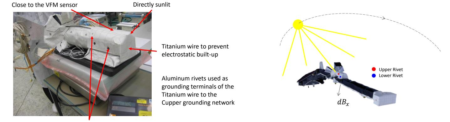
Thermal blankets grounded in both ends of the Titanium wire for redundancy
