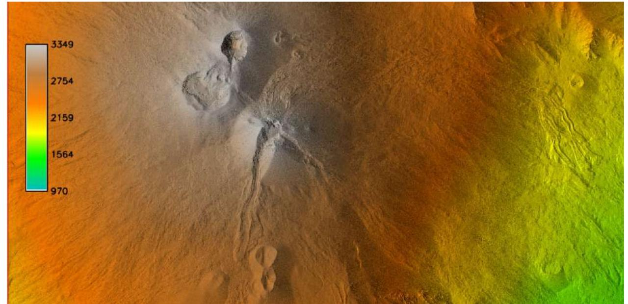
The 3D processing of the tri-stereo Pléiades imagery is performed using the free and open source MicMac (Multi-images Correspondances, Méthodes Automatiques de Corrélation) photogrammetric library developed by the French IGN (Institut Géographique National).
