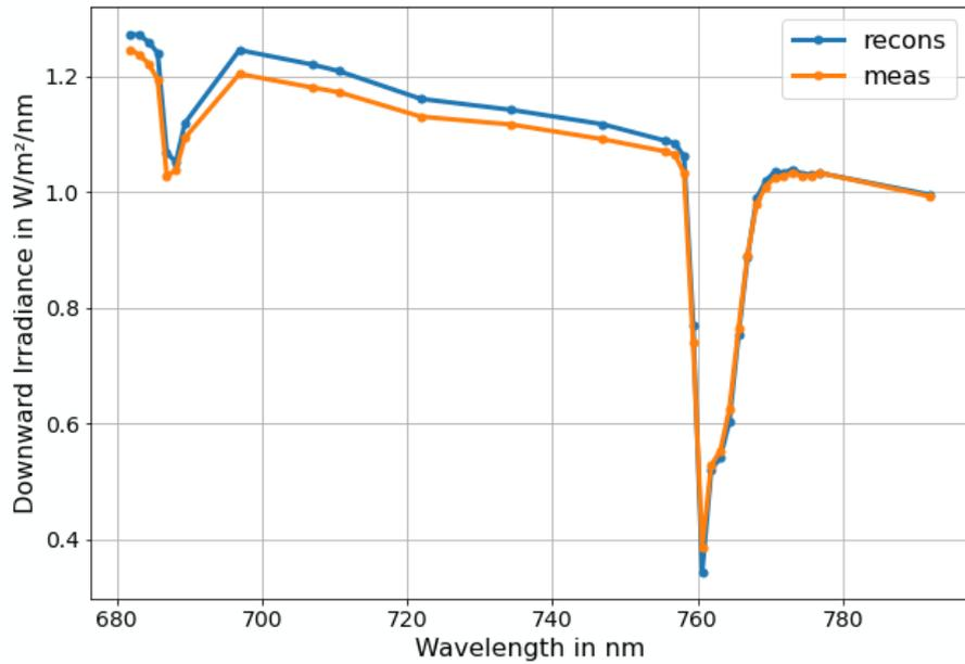
Fig. 5: FLOX spectrum of downward irradiance in OHP France 10/07/2018 and reconstructed from OLCI-FLEX.
