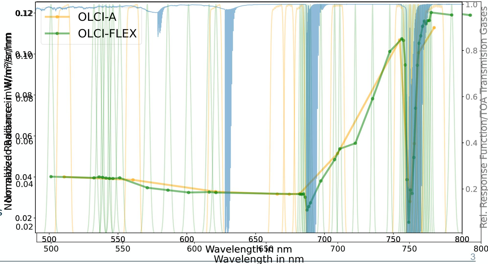
Fig. 2: TOA signal of OLCI-A and OLCI-FLEX with spectral response function in shaded colours and TOA transmission by atmospheric gases without H<sub>2</sub>O and O<sub>3</sub>
