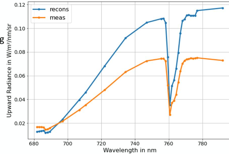
Fig. 6: FLOX spectrum of upward radiance in OHP France 10/07/2018 and reconstructed from OLCI-FLEX.
