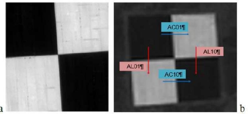
Figure 4-7-15-cm-Panchromatic-HD-(a)-artificial-MTF-target-in-Salon-de-Provence, 15-cm-Pansharpened-HD, and (b)-the-four-directions-(AL01, AL10, AC01, AC10)-of-the-MTF-calculation-(Red-band). $\eta$
