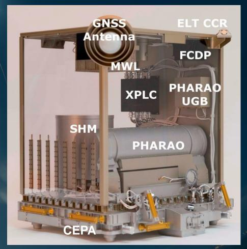
Volume: 1163x867x1153 mm<sup>3</sup> (plus ELT CCR and GNSS boom/antenna) Mass: 249kg plus CEPA (114kg) Power: 707W (typical)
