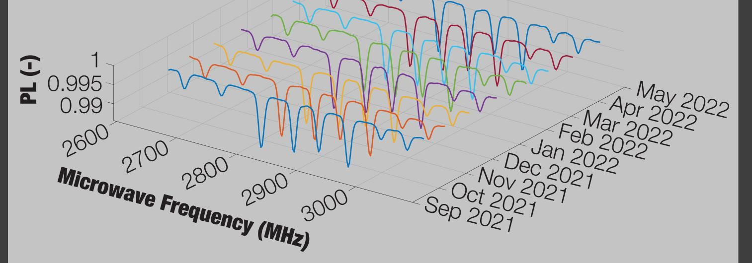
To assess the degradation of the OSCAR-QUBE sensor, measurements over a span of nine months were acquired. Normalized photoluminescence ODMR spectra with the eight peaks for comparison show no degradation, proving the feasibility of this technology in long-duration missions in space environment.
