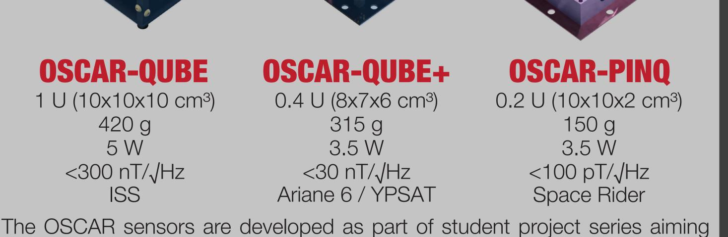
The OSCAR sensors are developed as part of student project series aiming at validating the viability of diamond-based sensors as a compact and stable sensing solution for future Earth Observation missions.
