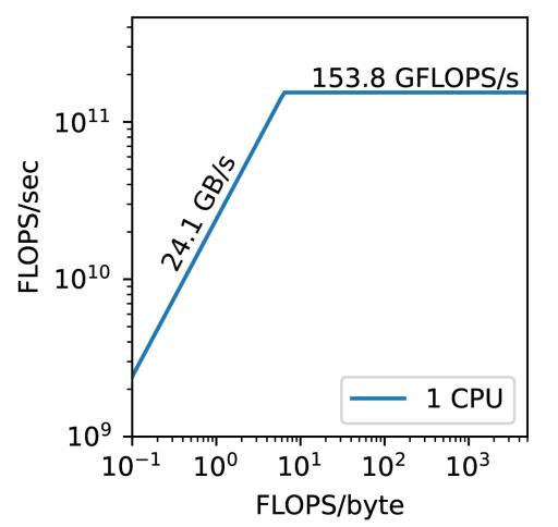
Measurements made via Empirical Roofline Tool
