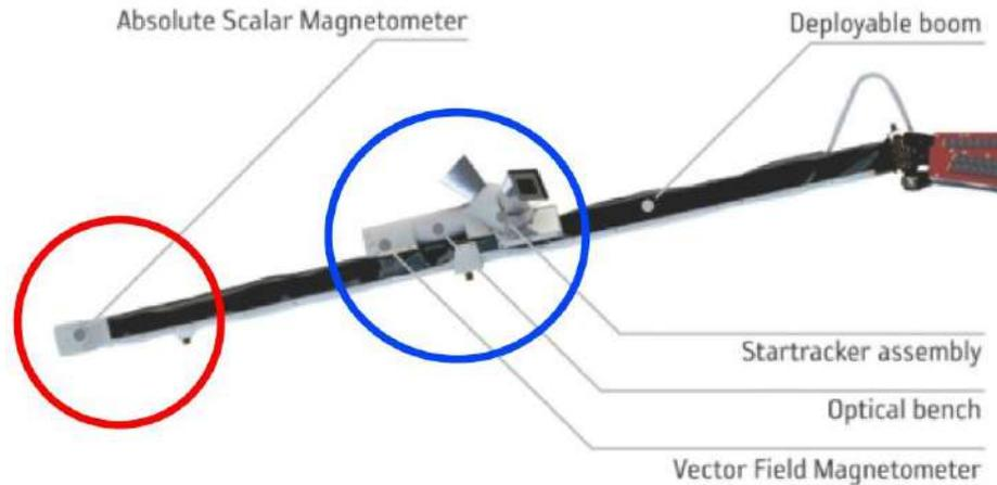
The ASM is first and foremost an **absolute scalar magnetometer** (based on atomic spectroscopy of  $^4\text{He}$ , and relying on the Zeeman effect)
