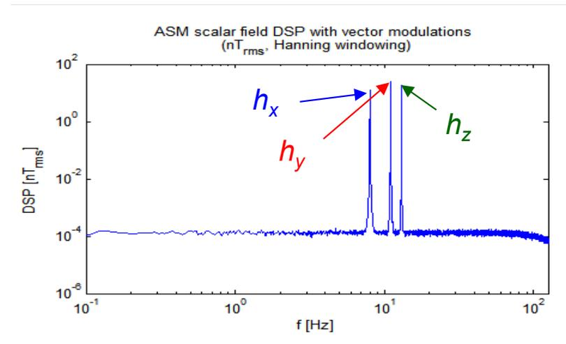
**The internal sampling** of the scalar sensors at **1kHz**, **allows** the instruments to be used in conjunctions with three sets of coils to also derive vector components at 1 Hz (**1 Hz “vector mode”**)
