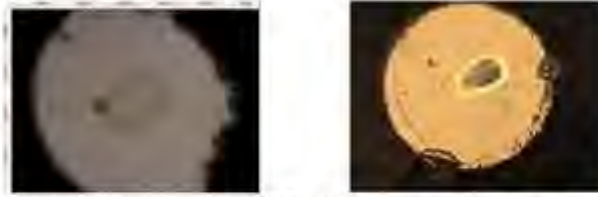
Fig. 1 (Left): An irradiated sample of C_6F_{13} (see green-yellow region in the center) as viewed between the diamonds with a microscope. (Right): After the sample was depressurized and released and the gasket material removed, a damage pit remained in the diamond surface etched by F_2 released during irradiation.
