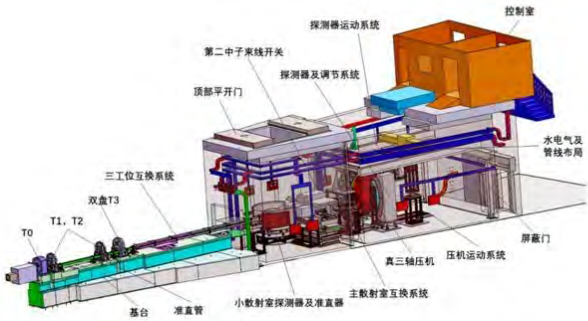
Figure 1. Schematics of the Integrated Neutron Diffractometer at Extreme Conditions (INDEC) at CSNS.
