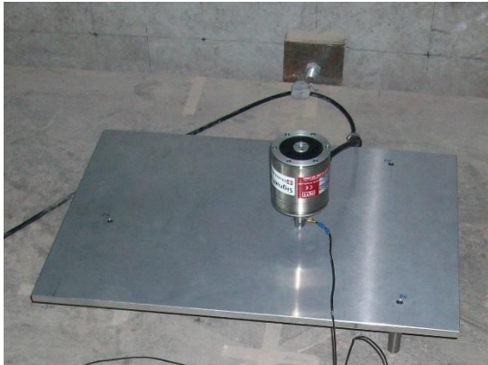
Figure 1: RRRS (Round robin reference source) on a low mobility reception plate (left); Reference Tapping Machine RTM (right); from [3].
