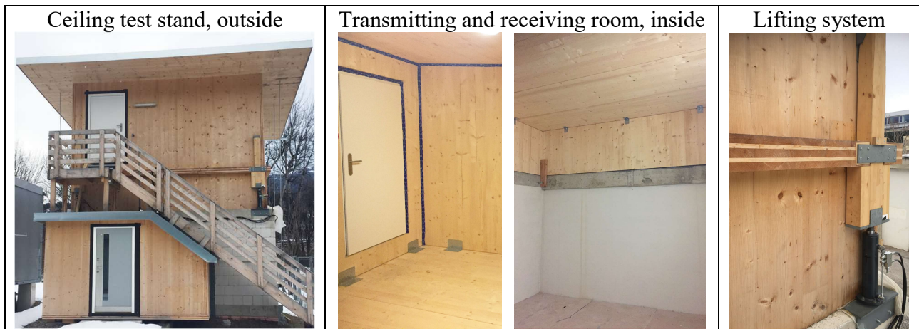
Figure 1: Acoustic ceiling test stand and detail images
