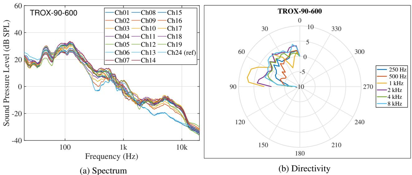
Figure 4: (a) Spectrum of the swirl diffuser from TROX measured with the 19 microphones of the microphone arc at a volume flow of  $600 \text{ m}^3/\text{h}$  and position  $90$ . (b) Directivity of the sound pressure level in dB SPL of the same air diffuser at the same room position as in (a), plotted for six one-third octave bands in reference to microphone No. 19 (at  $0^\circ$ ).
