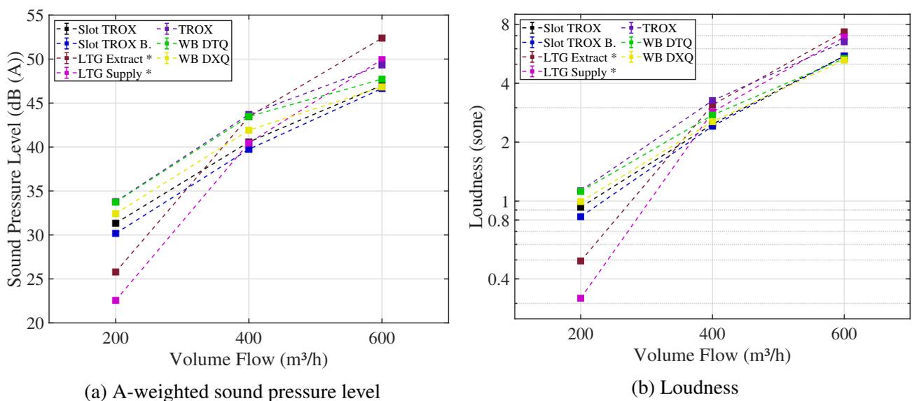
Figure 5: (a) A-weighted sound pressure level in dB and (b) loudness in sone over the volume flow for all measured air diffusers.
