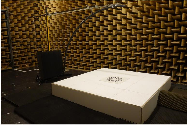
Figure 2: Measurement setup with the microphone arc in a hemi-anechoic room. The air diffusers were integrated into a ceiling tile construction.
