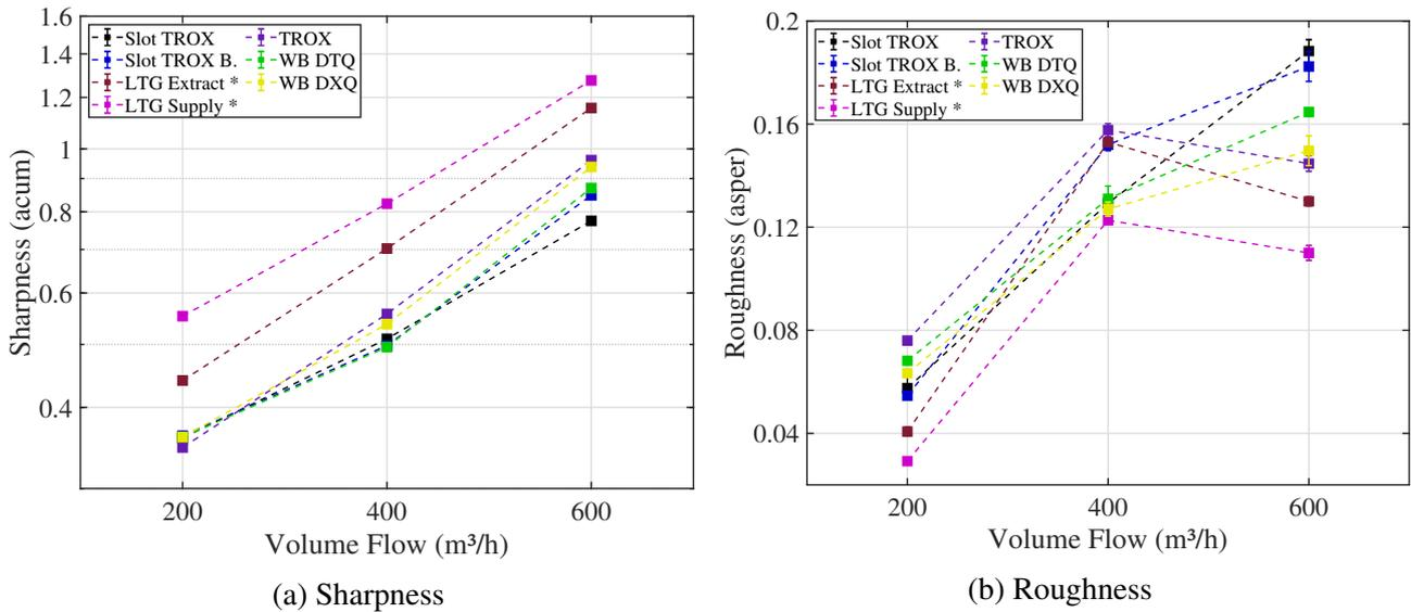
Figure 6: (a) Sharpness in acum and (b) roughness in asper over the volume flow for all measured air diffusers.
