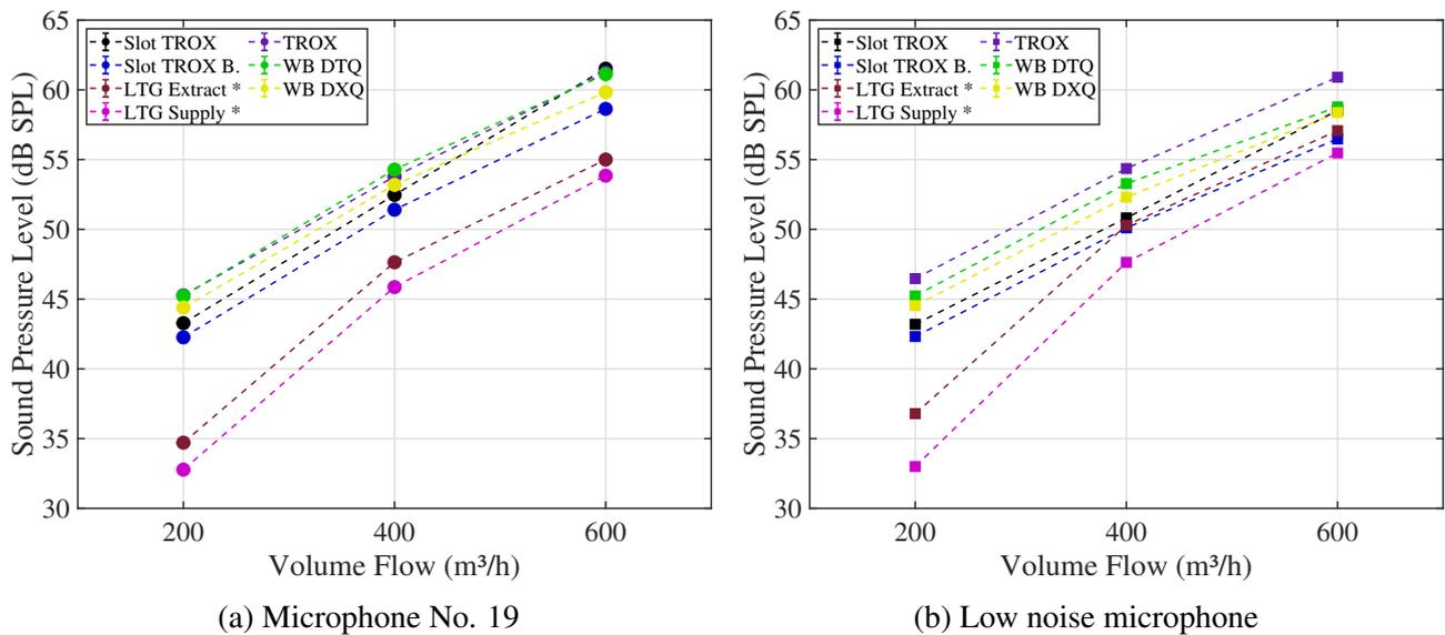
Figure 3: Comparison of the band-pass filtered sound pressure level in dB SPL between (a) the microphone No. 19 of the microphone arc and (b) the low noise microphone. They measured at the same position: centred 195 cm above the air diffusers.
