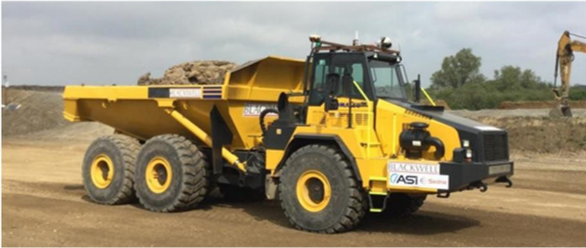
Figure 3: Trial of autonomous articulated dump truck on Highways England’s A14 Cambridge to Huntingdon Improvements scheme in 2018 (Photo copyright of Highways England and Blackwell Earthmoving Ltd).
