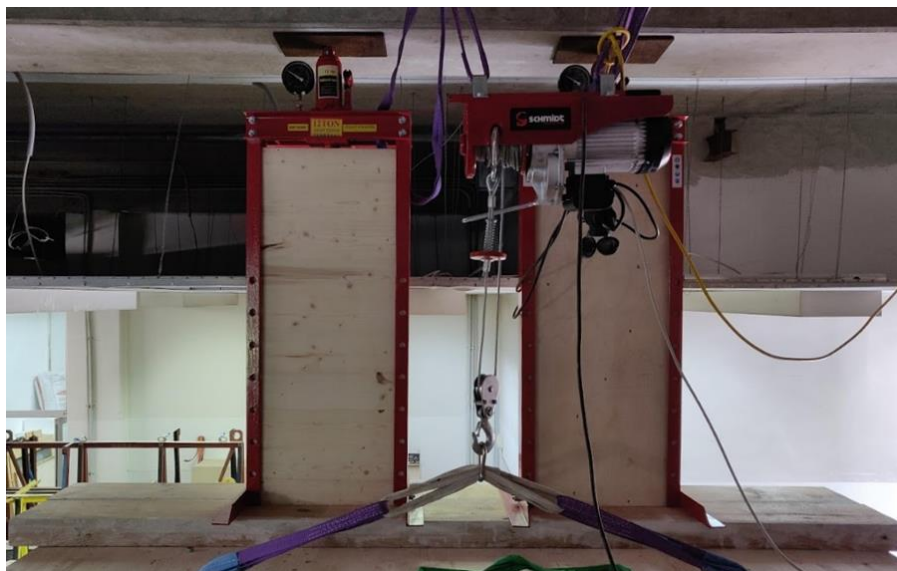
Figure 3: Device for pressing the element joint
