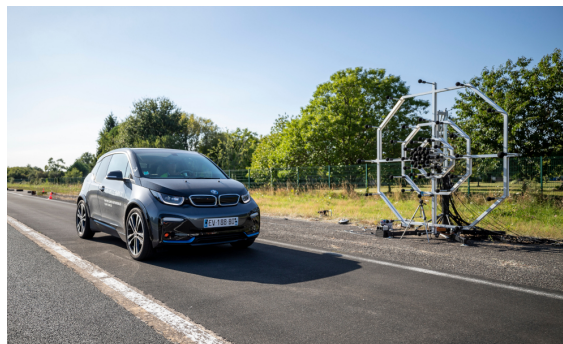
Figure 3: Microphone array and vehicle pass-by on road surface N
