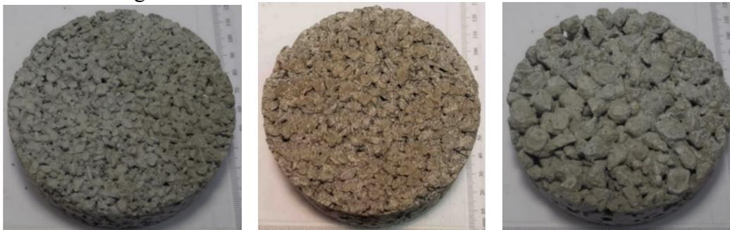
Figure 3: 25% porosity 100 mm diameter samples of PCC 0/4 (left), 0/6 (middle) and 0/10 (right).
