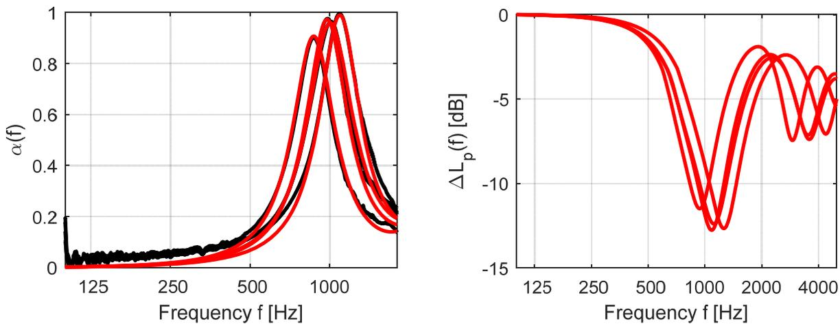
Figure 7: Measured (black curves) and predicted (red curves) absorption coefficient of PCC 0/6 samples (left) – Corresponding attenuation at roadside (right).
