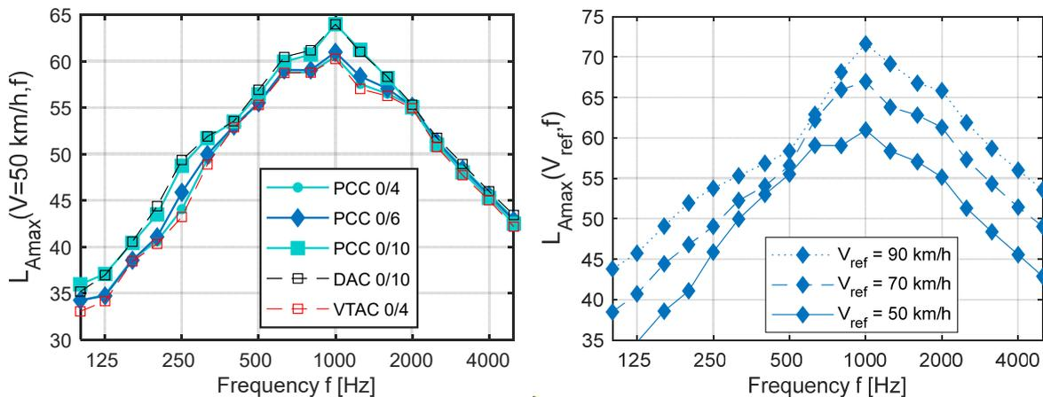
Figure 6: Predicted roughness induced noise spectra at 50 km/h for all PCC recipes (left) and for PCC 0/6 at 50, 70 and 90 km/h (right).
