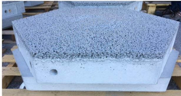
Figure 2: Precast slab with porous top layer.
