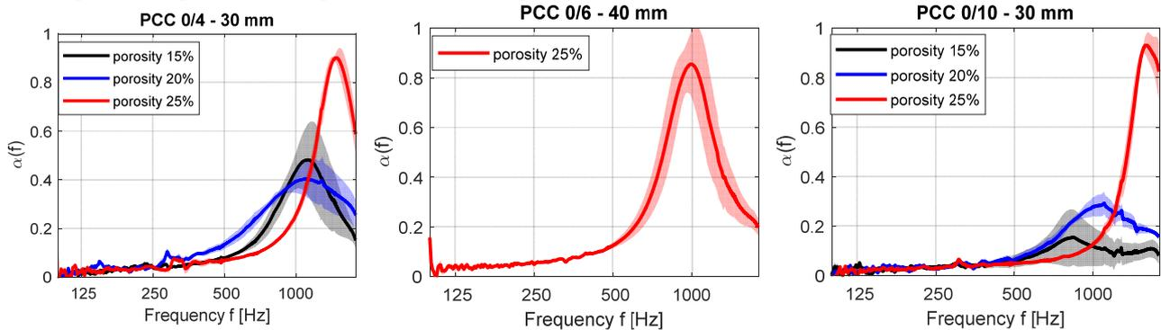
Figure 4: Absorption coefficients measured on 100 mm diameter PCC samples (with the variation range).
