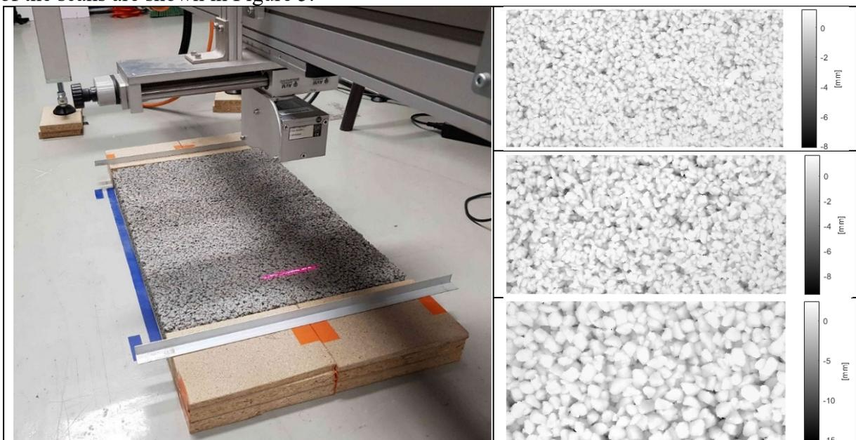
Figure 5: Scanning of a 40 cm by 60 cm PCC slab (left) – Extracts of 10 cm by 20 cm from scans of PCC 0/4, 0/6 and 0/10 (from top to bottom).
