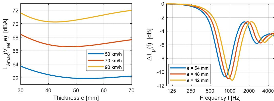
Figure 8: Predicted CB overall dBA noise levels versus porous layer thickness (left) - Attenuation due to absorption for optimal thicknesses (right).
