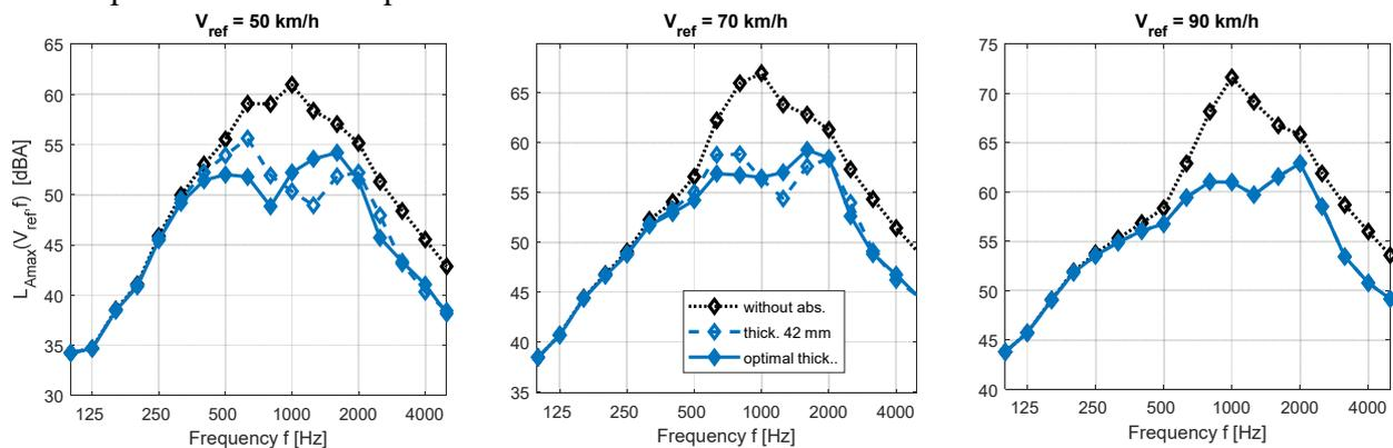
Figure 9: Predicted CB noise spectra for optimal thicknesses, for average PCC 0/6 samples thickness (42 mm) and without correction for absorption effect, for the three reference speeds considered.
