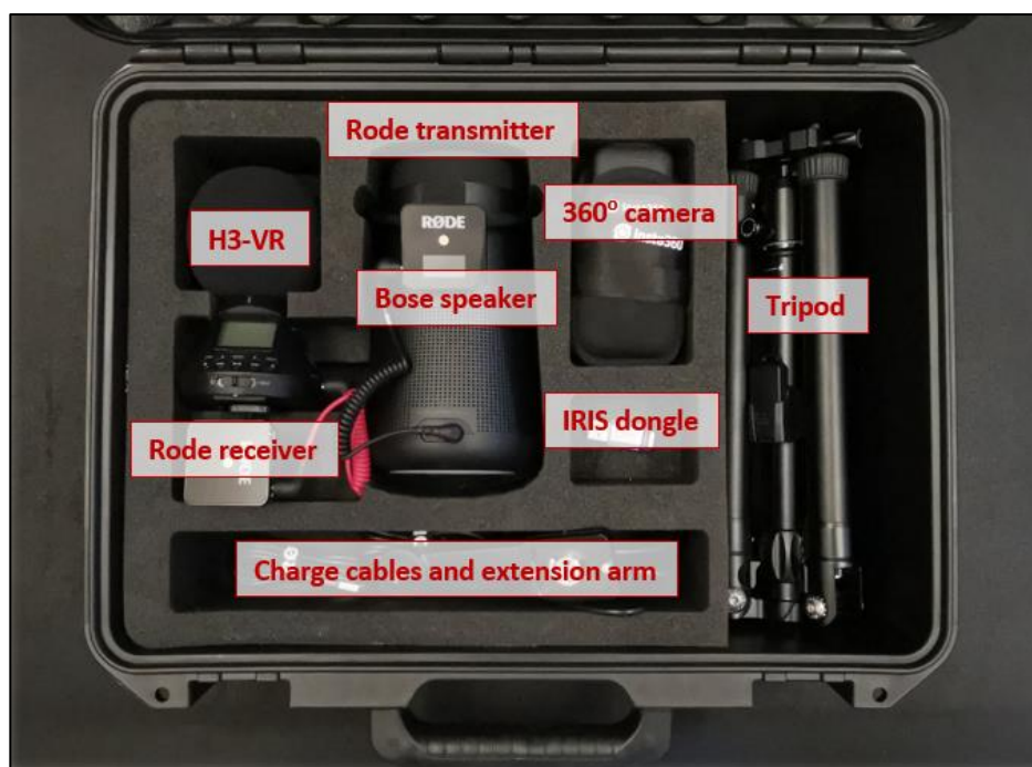
Figure 3: Mini IRIS kit in its case (laptop not shown)
