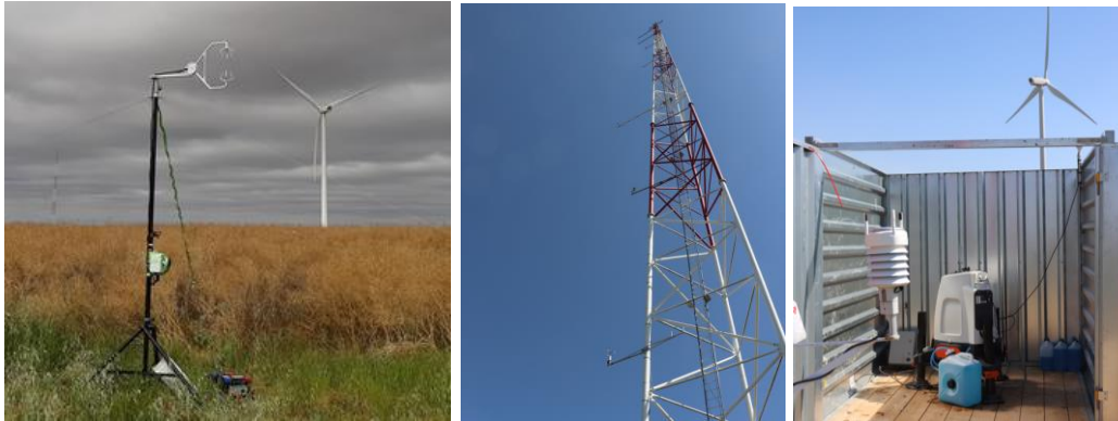
Figure 3: Meteorological apparatus. Sonic anemometer (left), meteo mast (middle), LIDAR (right)
