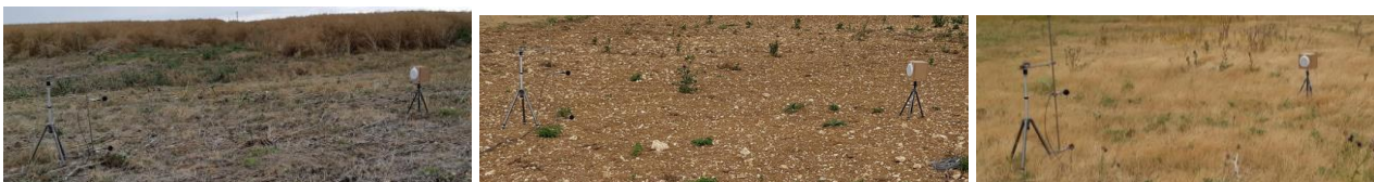
Figure 4: Experimental set-up for the measurement of ground acoustic impedance of three grounds
