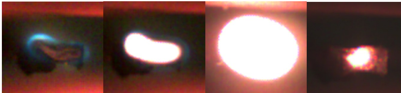
Figure 1. Images during the ignition and combustion of a biomass particle.
