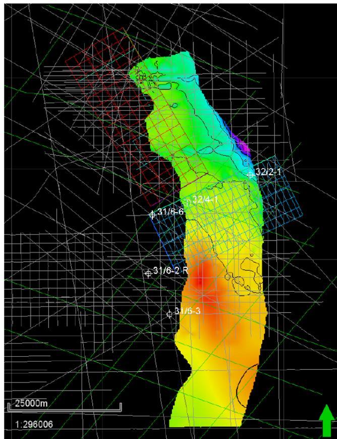
Figure 1: seismic and wells at Smeaheia. Blue and red grids give the location of respectively GN1101 and TNE01 3D cubes. The five wells are indicated by white crosses and the 19 2D seismic surveys in the area are also indicated.
